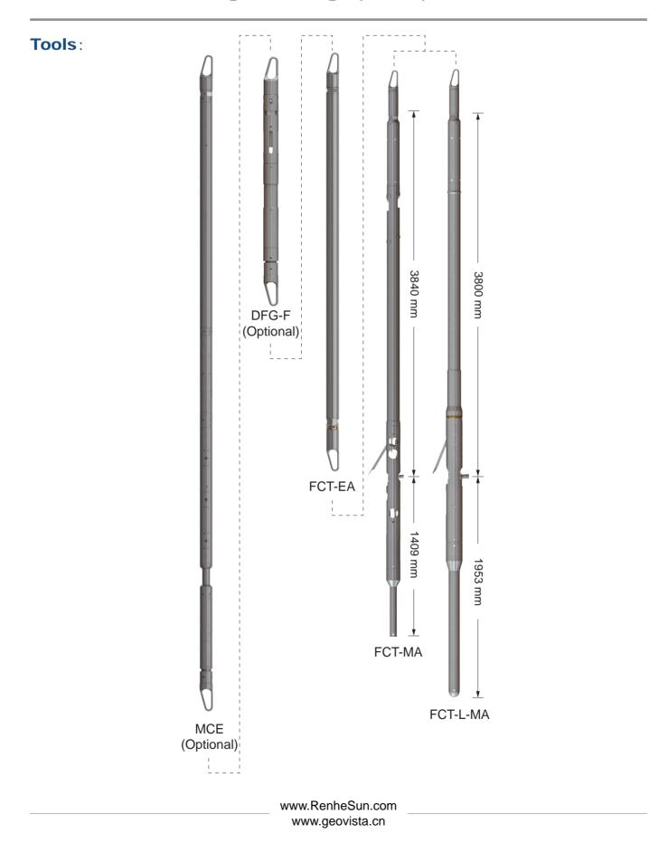
Large Core & Horizontal Formation Coring Tool (LHFCT)
